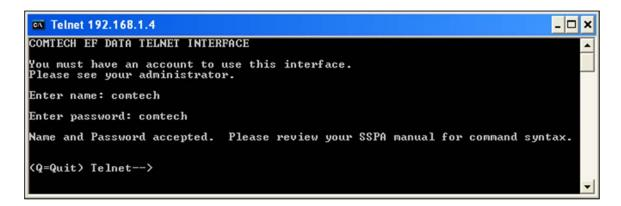
Once logged into the Telnet interface as the Administrator, you can access the standard remote control interface, defined in **Chapter 5. SERIAL-BASED REMOTE PRODUCT MANAGEMENT**, by typing in a pertinent remote command or query at the **Telnet -->** prompt.
