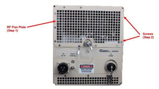
Figure 6-1. RF Fan Plate with Screws
