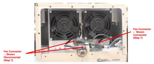
Figure 6-3. RF Fan Connectors
